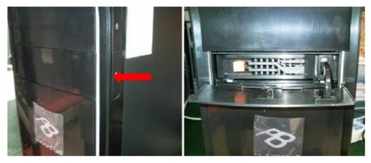
9.2 Press orange latch towards the right, open the handle and pull out HDD Carrier
